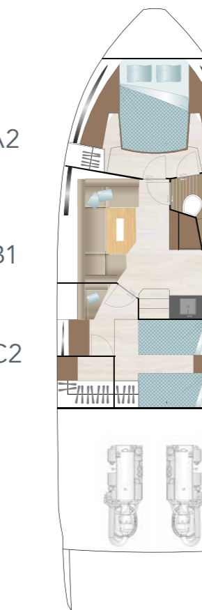
LOWER DECK Guest cabin with 2 single berths on starboard side and walk-in closet on portside option
